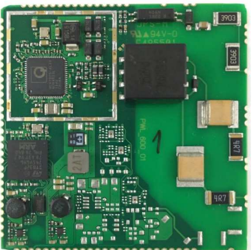
WHITE beet H Engineering Sample (without shielding)
