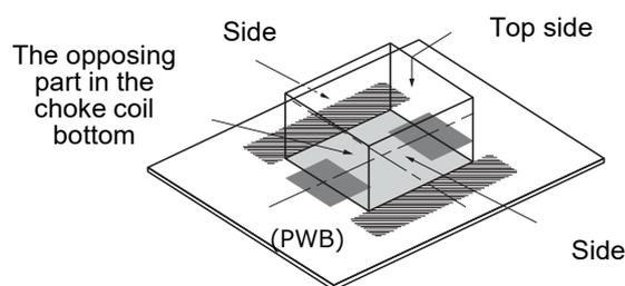
④ This power choke coil is different from the ferrite core-type that installs general concentration GAP. It has the leakage magnetic bunch distribution of the choke coil to the vertical direction. Please be cautious when using parts and circuit compositions which are easily affected by the leakage flux.
