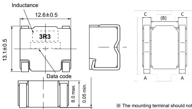
※ The mounting terminal should not protrude from C
