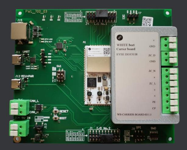
**WB-CARRIER-BOARD 1.1** is an evaluation and development board for WHITE-BEET 1.1 modules. It contains WHITE-BEET 1.1 module populated on the carrier board and protected with a plastic cover.
