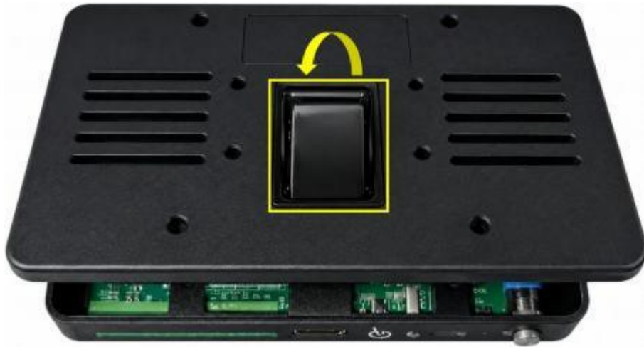
Figure 3-2 Rear Cover Latch Lever (lift upward to open)
