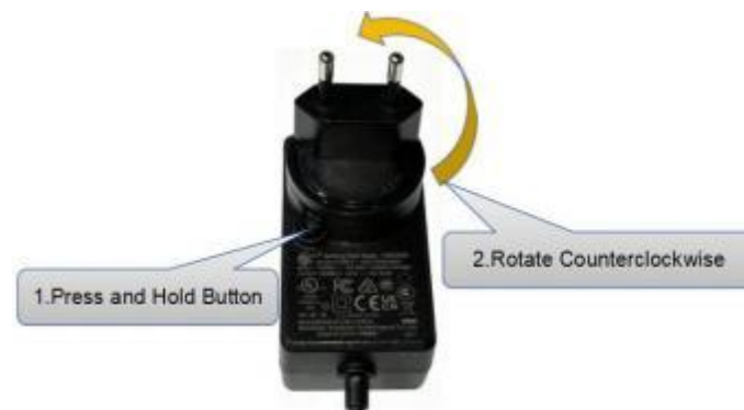
Figure 3-7 Power Adapter Plug Removal (press button + rotate counterclockwise)
