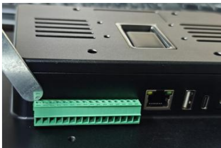
Figure 3-11 16-Pin Terminal Removal
