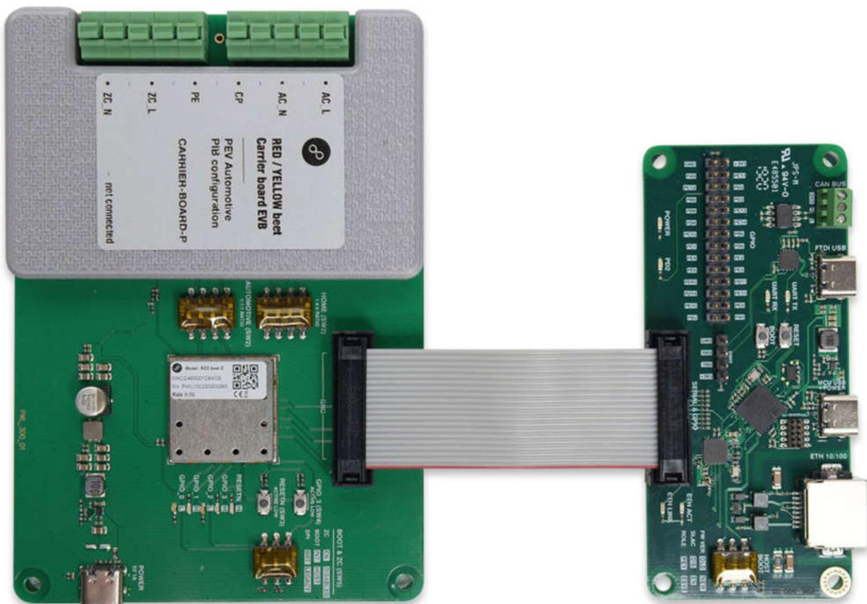
2. The second option to get control of CARRIER board is to use Raspberry Pi 3/4. You require a custom cable for that, please refer to the Table 2-1 for pinouts details.
