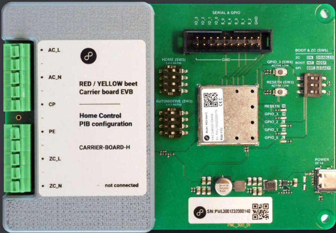
Carrier board allows testing and evaluation of RED and YELLOW beet modules in all applications starting from e-Mobility (EVSE and PEV) to other enterprise and home applications requiring long-range communication like smart grid, smart meter, IoT, home control and etc.
